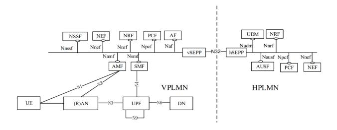
Figure 1: 5G Core Network Architecture.
