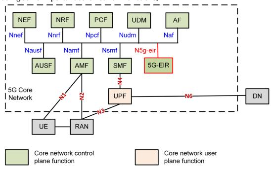
Figure 1: Service based architectural view of 5GS [Adapted from TSDSI STD T1.3GPP 23.501-17.6.0 V1.2.0]
