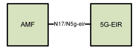
Figure 4: Non-roaming architecture for EIR Services in 5GS [Ref: TSDSI STD T1.3GPP 29.511- V18.1.0]
