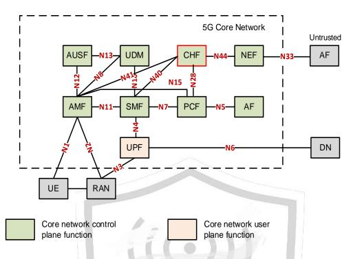
Figure 2: Reference point representation for 5GS [Adapted from: TSDSI STD T1.3GPP 23.501-17.6.0 V1.2.0]
