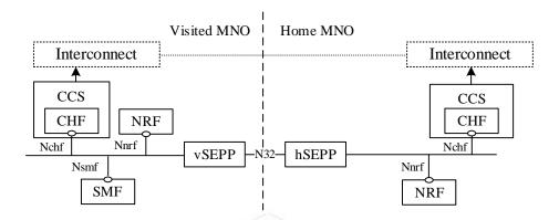
Figure 5: Roaming 5G data connectivity scenario in service-based interface representation: [Reference: 3GPP TS 28.827 V1.9.0 (2023-05) Release 17, "Study on 5G charging for additional roaming scenarios and actors"]
