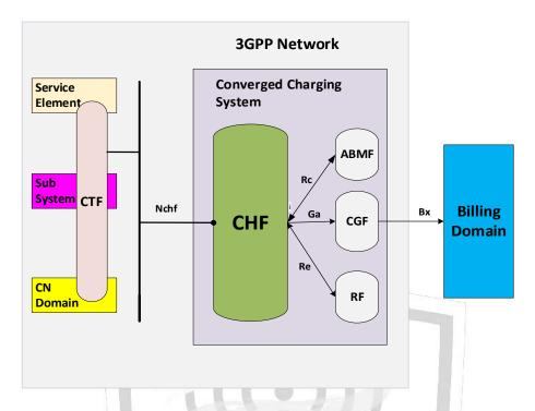
Figure 3: Logical ubiquitous converged charging architecture [Adapted from: Fig: 4.3.3.0.1 TSDSI STD T1.3GPP 32.240-17.8.0 V1.3.0]
