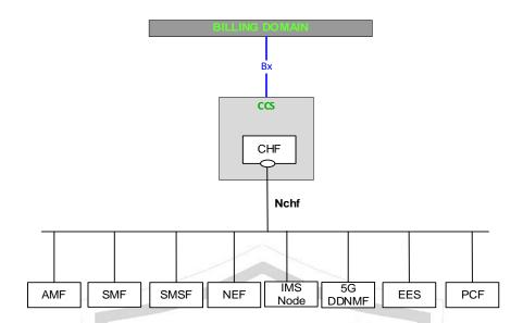
Figure 1: Logical ubiquitous charging architecture and information flows for 5G systems – service-based representation [Reference: Fig:4.2.3.1 TSDSI STD T1.3GPP 32.240-17.8.0 V1.3.0]
