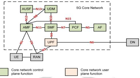
Figure 2: Reference point representation for 5GS [Adapted from: TEC 26065:2022/TSDSI STD T1.3GPP 23.501-17.6.0 V1.2.0]
