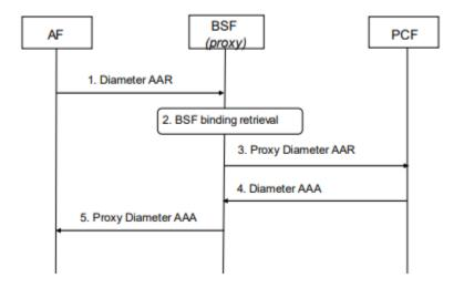
Figure 7: Rx Session establishment procedure using BSF proxy [Reference: 3GPP TS 29.513 V17.0.0 (2020-09)]
