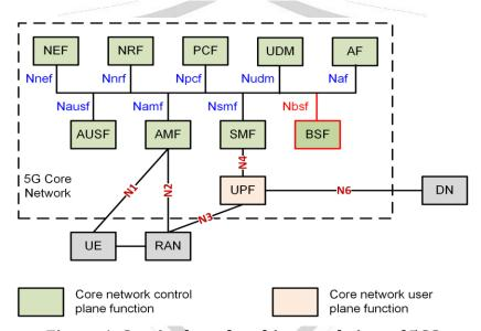
Figure 1: Service based architectural view of 5GS [Adapted from: TEC 26065:2022/ TSDSI STD T1.3GPP 23.501-17.6.0 V1.2.0]
