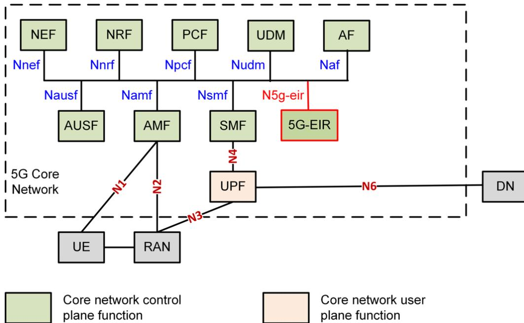
**Figure 1: Service based architectural view of 5GS**
